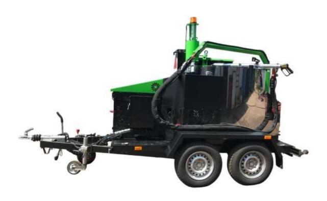
Crack sealing machine BPM-500 is used for sealing cracks, seams and waterproofing, as well as for repair and construction works on roads with the use of bitumen-elastomeric sealing mastic. Specially designed sleeve fastening system, which significantly reduces the likelihood of its failure.
